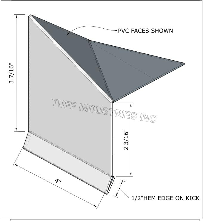
TD-20 METAL DIVERTER SADDLE FLASHING
