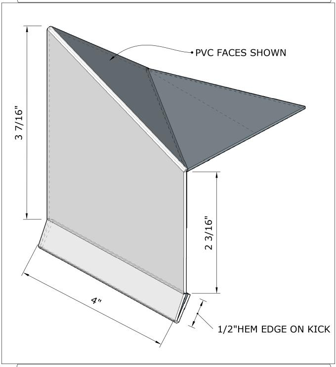
TD-20 METAL DIVERTER SADDLE FLASHING
