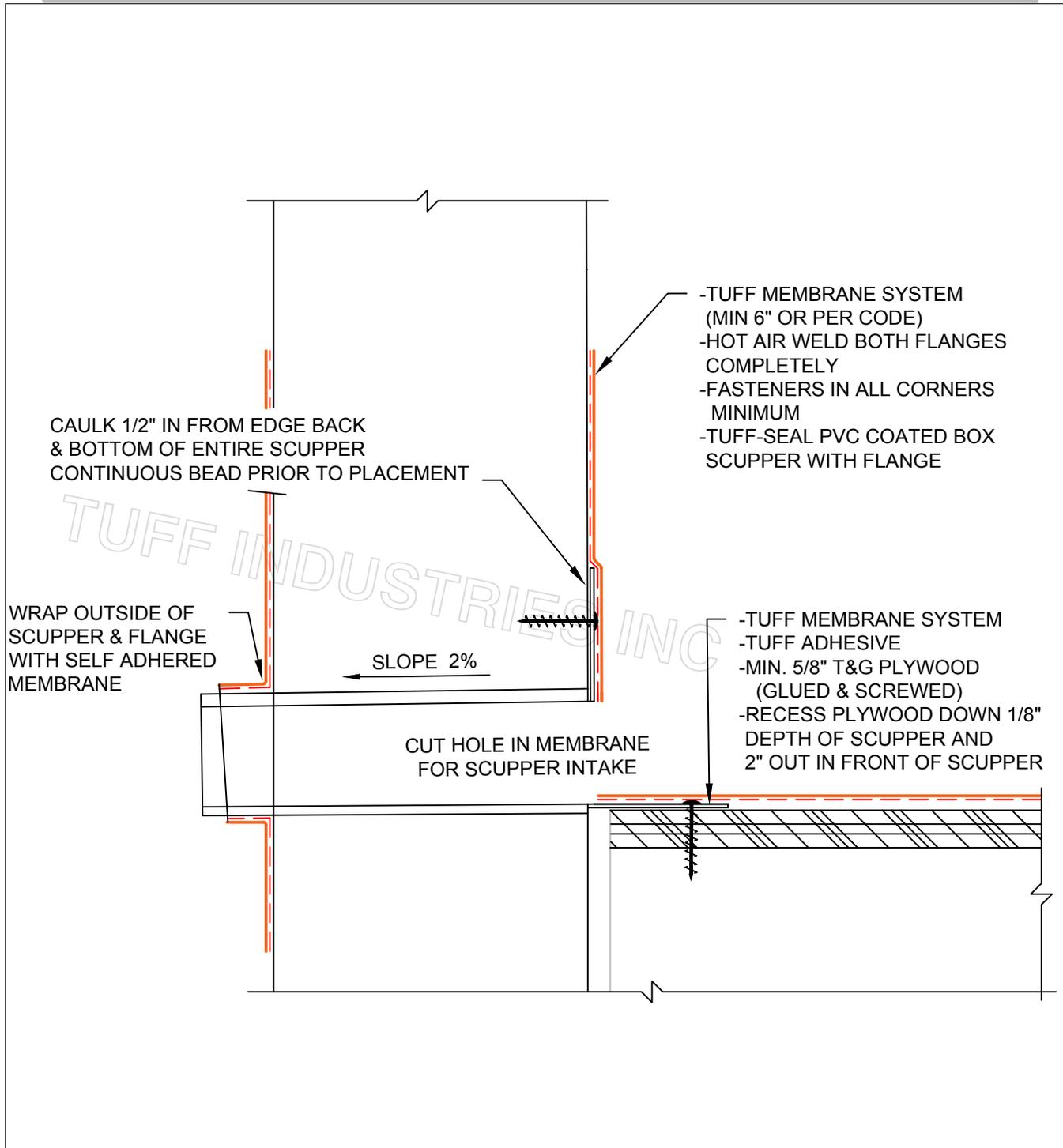
**TD-22A TUFF-SEAL PVC BOX SCUPPER WITH FLANGE INSTALL**
