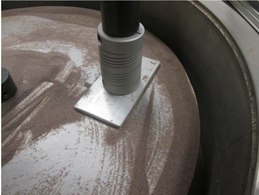
Representative Close-up of Sample in Abrasion Tester
